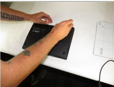
Unscrew the four (2.5 mm Phillips) screws (Use Phillips #0 Screwdriver).
