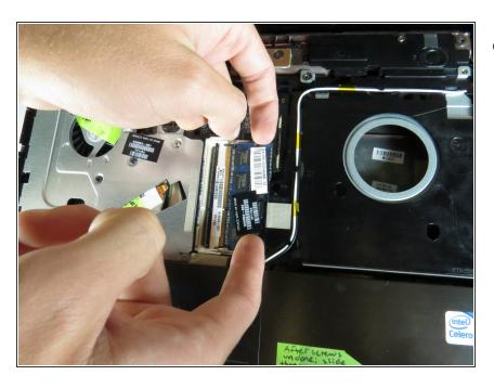
Press the two prongs outward, and the RAM card will come out of PCI Express connector.
