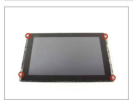
Remove the four 2 millimeter Phillips #00 screws at the corners of the tablet.
