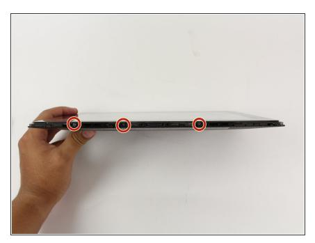
Use a Phillips #00 Screwdriver to remove the three 3 millimeter screws securing the front panel to the back panel found on the bottom portion of the tablet near the port.
