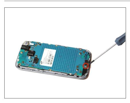
Remove one Phillips 3.93 mm screw from the bottom center of the phone.
