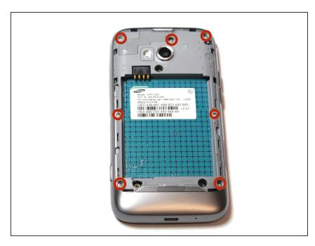
Remove the 7 Phillips 3.93 mm labeled screws by using the Phillips #00 Precision Screwdriver.
