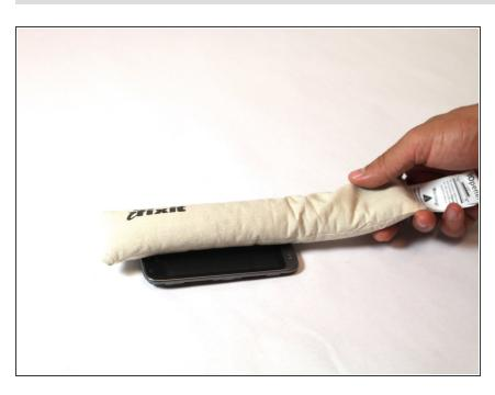
• Heat iOpener in microwave for one minute on the highest power setting. Let the iOpener sit on the device for about 90 seconds. This step is necessary to loosen the glue under the display screen. Be careful, the glue is very sticky!
