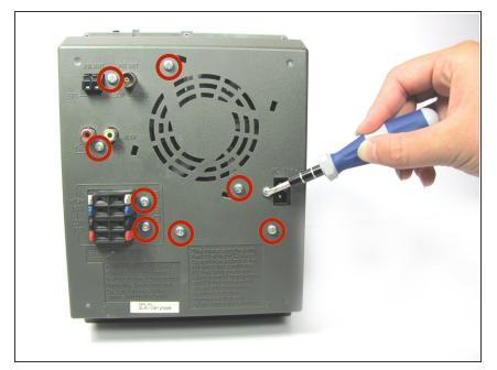
Remove the eight 9.5 mm #2 Phillips screws attaching the back to the device.
