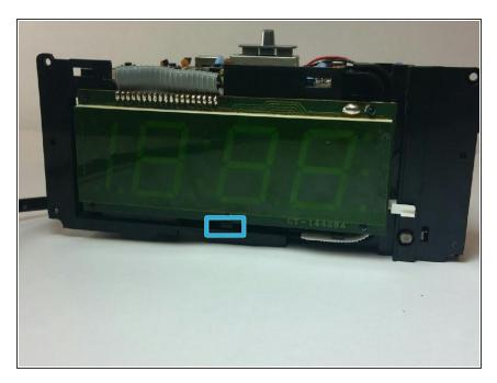
First release the latch highlighted in the picture. Then grab the screen by the bottom and lift it up.
