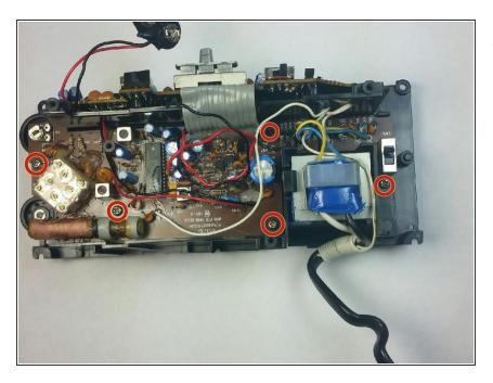
Remove the 5 10mm Phillip's #1 screws that holding side part of the motherboard
