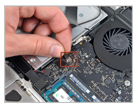
Disconnect the camera cable by pulling its connector away from the socket (toward the optical drive) on the logic board.
