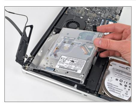
Lift the optical drive near its connector and pull it away from the upper case to remove it from the computer.
