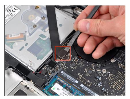
Use the flat end of a spudger to pry the AirPort/Bluetooth ribbon cable connector up off the logic board.
