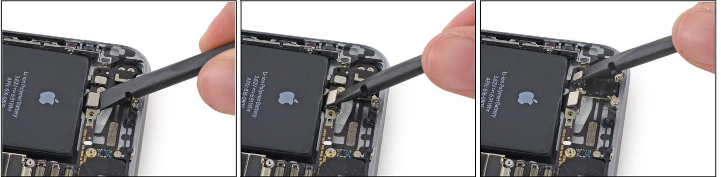
⚠ When disconnecting the following connectors, only pry up on the connector, **not the socket** on the logic board or you risk permanent damage.
