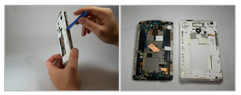
• Use the small plastic opening tool to pry between the screen and the rear case.
