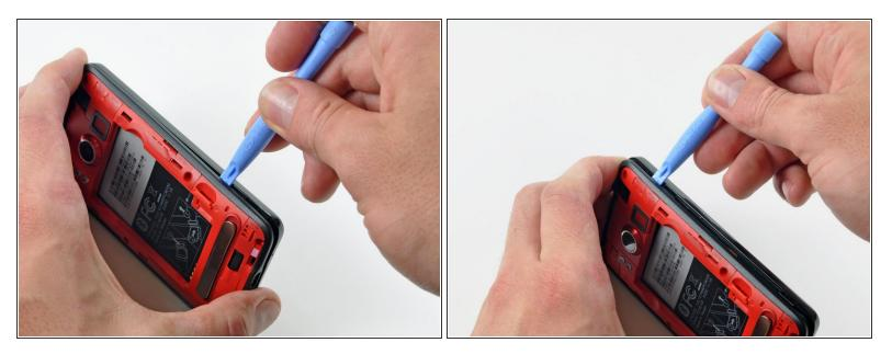
Insert the iPod opening tool between the rear inner frame and its plastic surround and pry up at several points along the left edge of the Evo.
