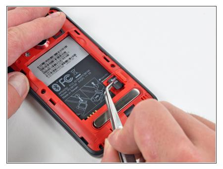
• Use a pair of tweezers to carefully pull the MicroSD card out of its slot in the inner rear frame.
