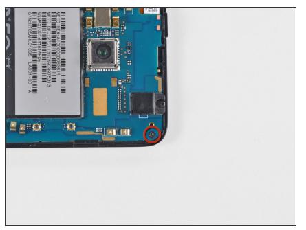
Remove the single Phillips screw securing the motherboard to the inner case near the headphone jack.
