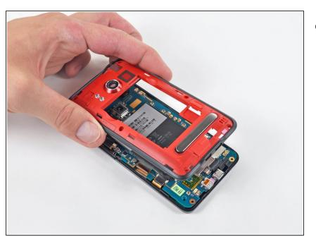
Remove the rear inner frame from the rest of the Evo.
