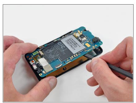
• Use the flat end of a spudger to pry the motherboard off the posts securing it to the metal display tray.
