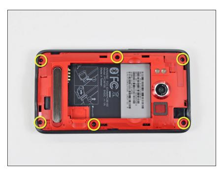
Remove six T5 Torx screws securing the rear inner frame to the inner case.
