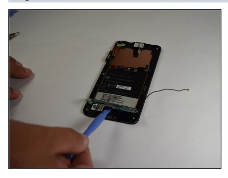
Using the plastic prying tool, pry the PCB device from the screen of the phone.
