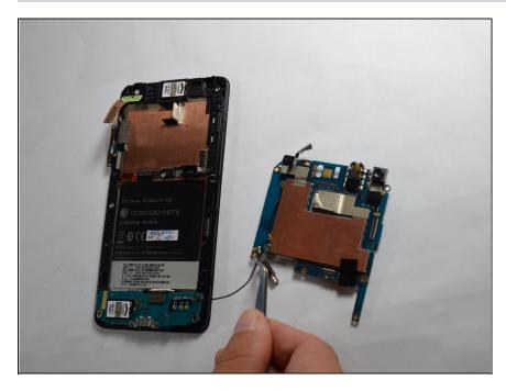
Disconnect wire going from the printed circuit board to the motherboard using the tweezers.
