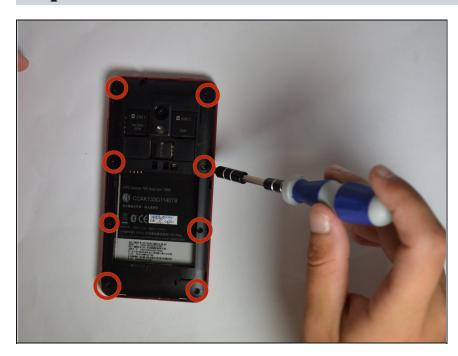
• Remove eight 8.3mm T4 screws with the Torx screwdriver.
