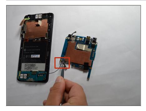
• Unsnap the wire from the printed circuit board (PCB) using the tweezers.
