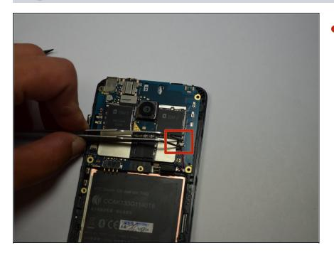
Using the <u>tweezers</u> gently disconnect the wire from the vibrator located on the motherboard.
