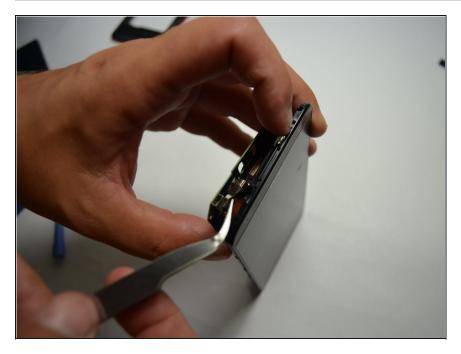
• Carefully remove the ribbon attached to the top of the motherboard.
