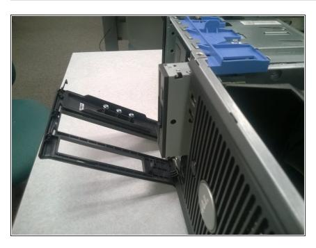
To remove the unconnected floppy drive from the drive bay, slide the drive towards the front of the computer.
