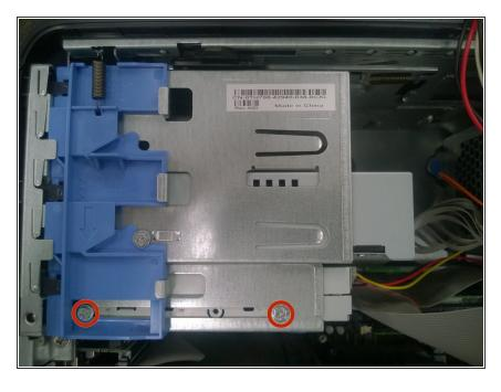
With a Phillips #1 screwdriver, remove the screws connecting the floppy drive to the drive bay. Set the
