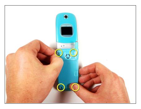
Using a thumb-tack, push-pin, or similar pin, remove the four plastic stoppers located on the back panel.
