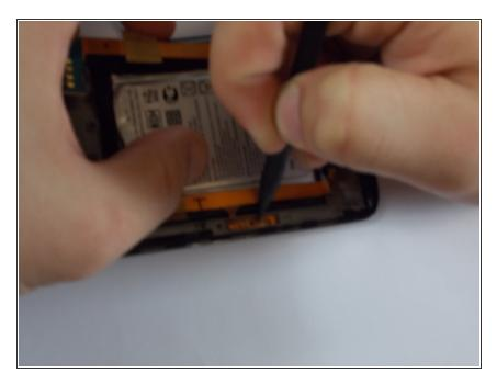
• Make sure you pay attention when removing the left flex cable because it is also connected to the side. Simply just peal this part away also. It may be a little more difficult than the upper connections, but just peel away. It may bend a little but be careful not to break.
