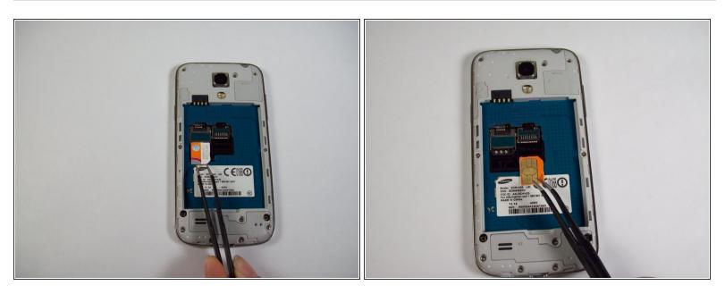
• Using tweezers, remove the SIM card by sliding it towards the bottom of the device.
