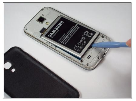
• Pry the battery out using a plastic opening tool.
