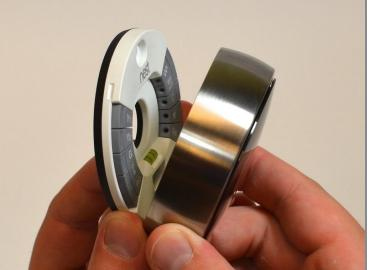
• Grasp the display's metal outer ring with your fingers and pull directly away from the wall.
