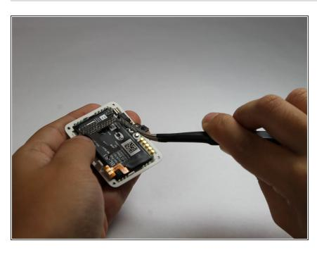
Use a pair of tweezers to gently lift the metal retaining clip up and out of the way.
