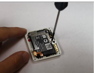
Remove the two black Phillips #000 2.5x3mm screws that are located on the right side of the metal clip.
