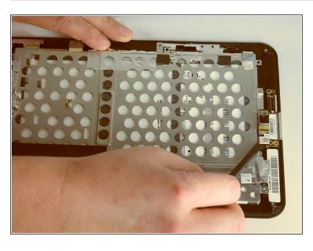
With a spudger, disconnect the cable connecting the camera to the motherboard.
