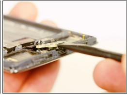
Now that we have access to the usb port, we use the flat end of or spudger and lift it off of its connector and free it from the daughterboard.
