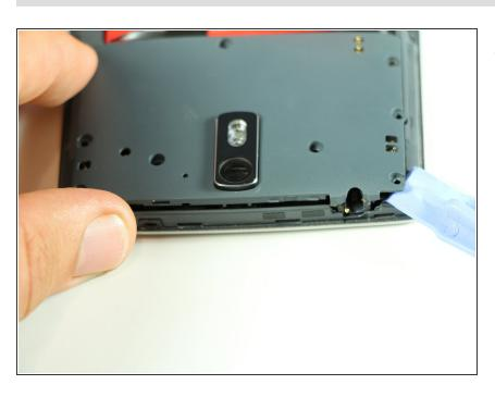
Using a plastic opening tool, gently pry up the black plastic cover and remove it from the device.
