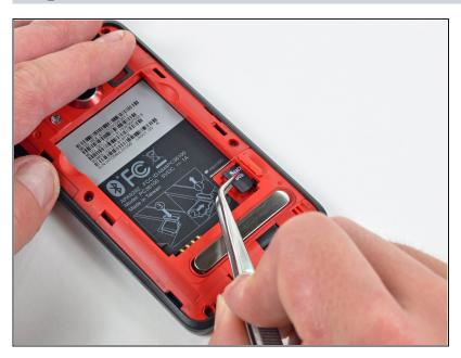
Use a pair of <u>tweezers</u> to carefully pull the MicroSD card out of its slot in the inner rear frame.
