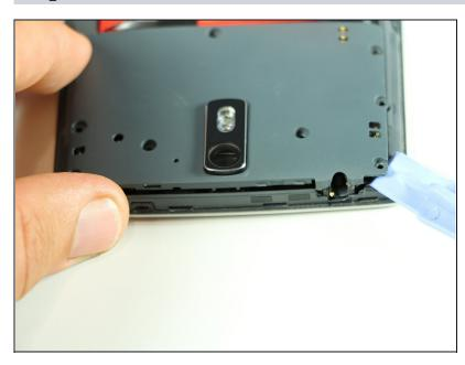
Using a plastic opening tool, gently pry up the black plastic cover and remove it from the device.
