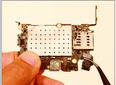
• Once the motherboard has been removed simply pry the front facing camera off of its connector with a spudger or angled <u>tweezers</u>.
