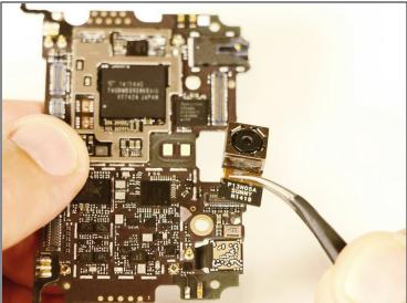
• Once the motherboard has been removed simply pry off the rear facing camera with a spudger or angled <u>tweezers</u>.
