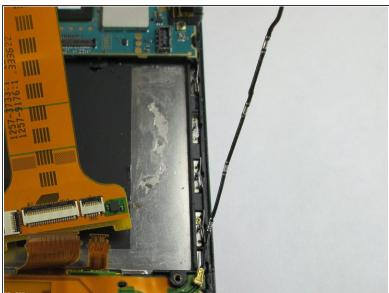
Use the plastic opening tool to unlatch the cord's ends off the motherboard and loud speaker module. The cord can be located on the right side of the phone.
