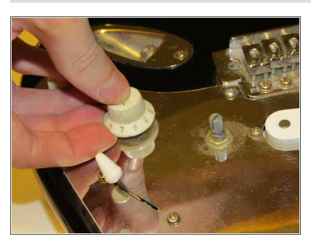
While it is not necessary to remove the potentiometer knobs in order to remove the pickguard, it is much
