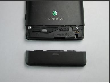
Use the plastic opening tool to pry the bottom plastic section off.
