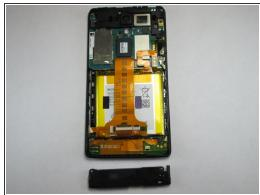
Use the plastic opening tool to remove the loud speaker module.
