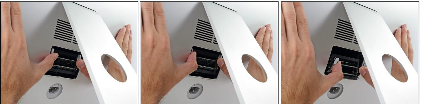
ⓘ The RAM tray is locked into its upright position with two grey tabs.
