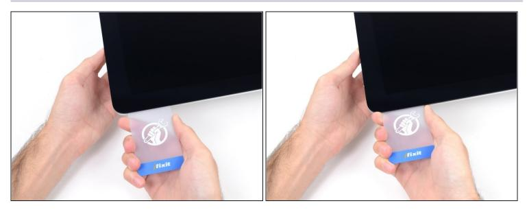
• Put the card into the corner again and let it stay there to keep the adhesive from resettling.
