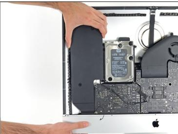
• Lift the left speaker straight up, until the power button cable is exposed (about 0.5 inches).
