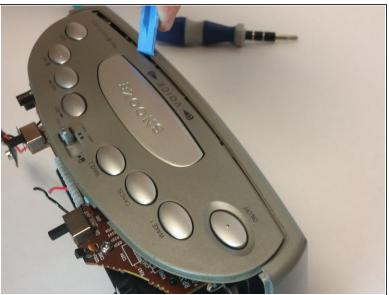
Pry open both tabs to remove the topside of the clock.
