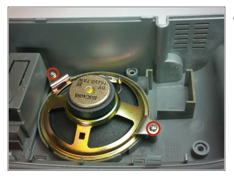
Remove the two 10mm Phillip's #1 screws. Also remove the two reinforcements holding the speaker in place.
