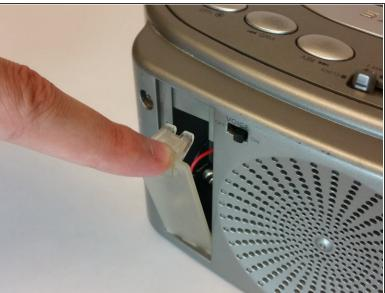
Push down on the clip to release pressure. The pull off the plastic cover.
