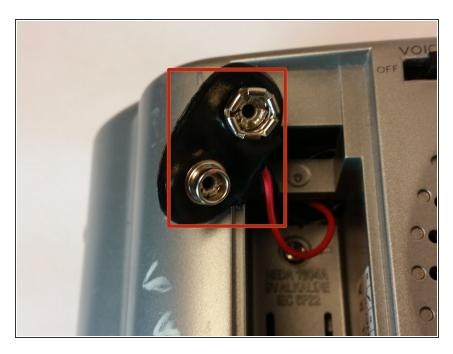
Remove the 9-volt battery from the battery terminal.
