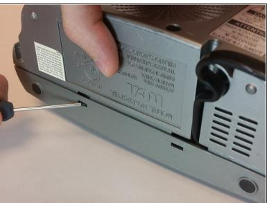
Using flathead screwdriver undo the release tabs.
