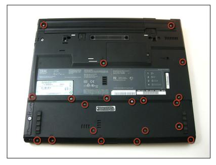
Using a Phillips #0 screwdriver, identify and unscrew the twenty screws located on the underside of the T42.
