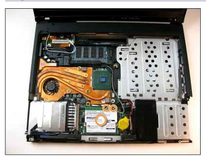
To remove Wi-Fi card, first disconnect both display wires on the top right.
