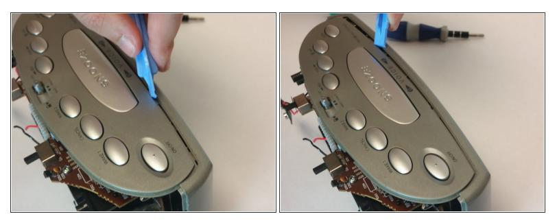
Pry open both tabs to remove the topside of the clock.
