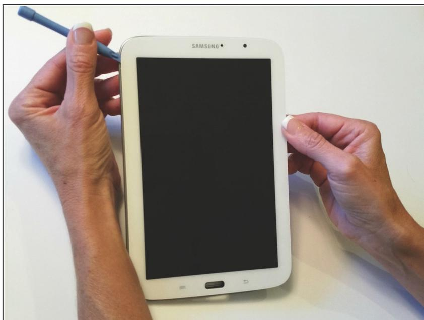
**⚠** When inserting your opening tool on the side opposite the power button, avoid the screen cable located 7 cm from the top of the device.
