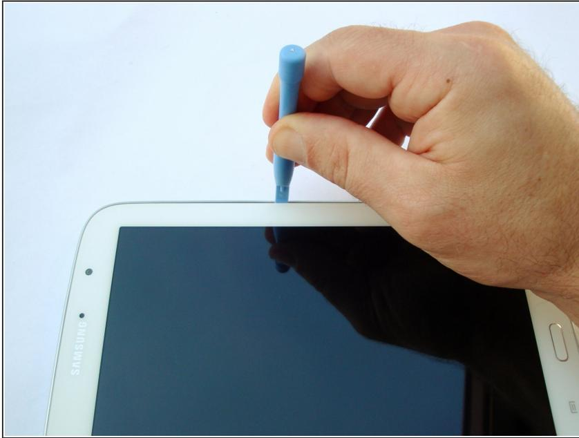
**⚠** It is important that you separate the 3 edges only at this time. The side of the tablet opposite the power button has a connection that could be damaged if this side is separated.
