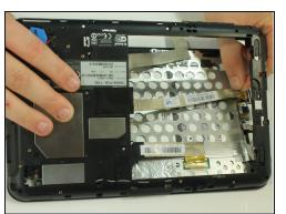
• Once the back of the case is off, disconnect the wires by gently pulling on the plastic tabs as shown.
