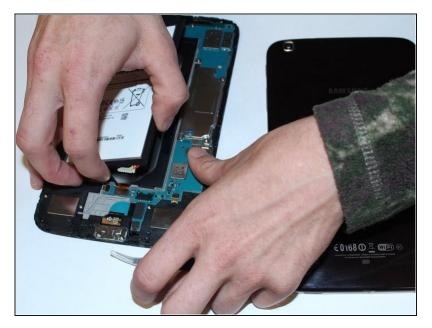
After the battery is disconnected, use the pulling tab to safely remove the battery.
