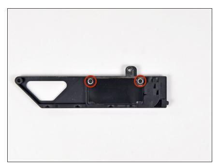
Remove the two Phillips screws securing the AirPort/Bluetooth board to the AirPort/Bluetooth board housing.
