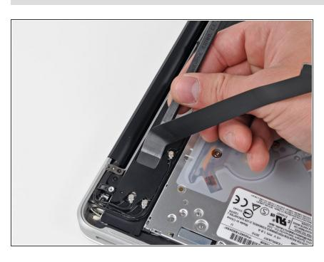
Use the flat end of a spudger to pry the AirPort/Bluetooth cable connector up off its socket on the AirPort/Bluetooth board.
