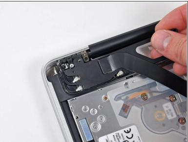
Before securing the AirPort/Bluetooth bracket to the upper case, be sure the small plastic tab on its left edge is inserted into the small void cut into the black plastic optical drive opening.
