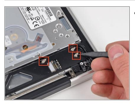
Pry the AirPort and Bluetooth antenna connectors (3 total) up off the AirPort/Bluetooth board.
