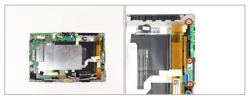
Use a Phillips #00 Screwdriver to remove the three 3 millimeter screws securing the buttons to the back panel.
