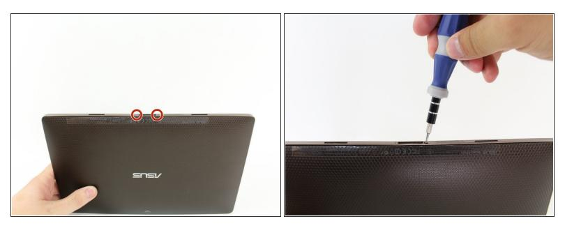
Use T5 Torx Screwdriver to remove two 4.5 millimeter T5 screws on either side of the port on the bottom of the tablet.
