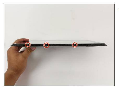
Use a Phillips #00 Screwdriver to remove the three 3 millimeter screws securing the front panel to the back panel found on the bottom portion of the tablet near the port.
