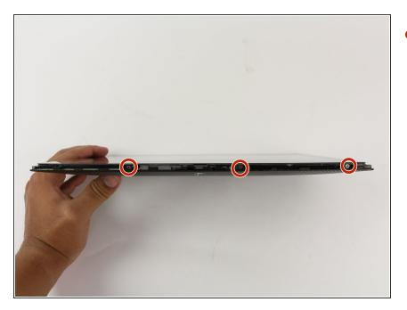
Use a Phillips #00 Screwdriver to remove the three 3 millimeter screws securing the front panel to the back panel found above the camera area, on the top portion of the tablet.
