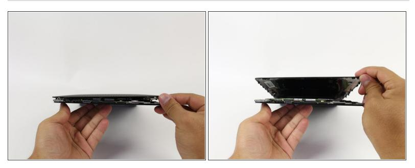
• Remove back panel by pulling away from the remaining device.
