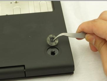
• Using a pair of tweezers, remove the two rear rubber feet to expose two hidden screws.
