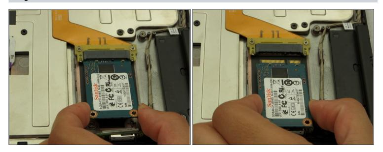
• Firmly grasp the SSD with two fingers slightly upwards and pull.
