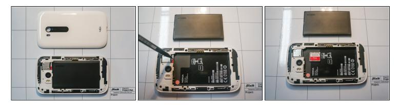
• Remove the back cover, the battery, and the sim card with its bracket.
