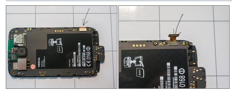
• Locate the ribbon cable on the back of the logic board and carefully loosen the connector with a plastic opening tool. Be sure you are prying on the cable's connector, and not on the plug on the logic board.
