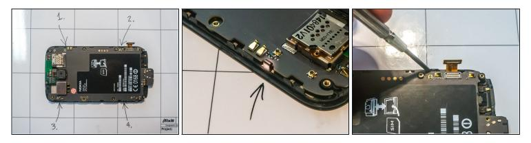
There are four small plastic clips that hold the logic board to the screen assembly. Using a small flat screwdriver, carefully pull back clips # 1 and 2, (see photo) and free the logic board on that side.
