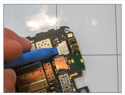
On the logic board, the front facing camera, along with the proximity and light sensors can be removed simply by loosening the connector with a plastic opening tool.
