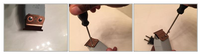
• Remove the two blade screws from the top blade of the trimmer.
