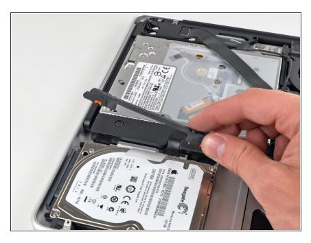
Lift the the retaining bracket out of the upper case.
