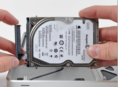
Remove the hard drive cable by pulling its connector straight away from the hard drive.
