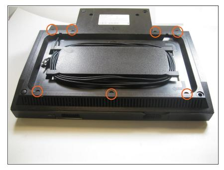
Flip your Atari Entertainment System over to its top so you can see the bottom. You'll see seven screws holding your system together. Use a Philips #0 screwdriver to remove all seven screws.
