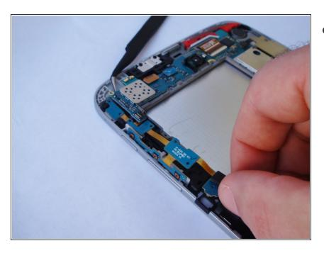
Hold the corner of the motherboard up and carefully slide the cable out.
