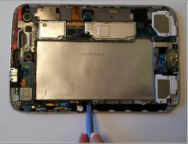
Gently pry the lower edge of the cable off the plastic stud just above the stylus opening.
