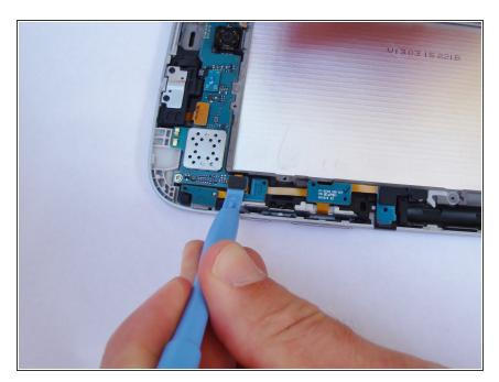
Disconnect the black connector by pulling up using a plastic opening tool underneath the edge. This connection attaches the power/volume cable to the mother board.
