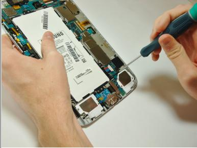
Remove the 8 Phillips#00 3-mm screws holding the battery in place.
