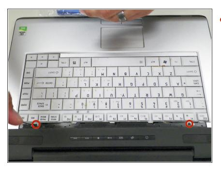
Remove 2 Phillips 3.1 mm size screws from each side above the keyboard.
