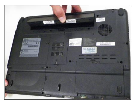
Gently lift and pull the battery out of the device.
