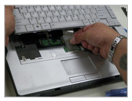
Gently lift keyboard a few inches above device, exposing the attached ribbon cable.
