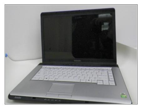
Turn the device so the top side is facing up. Open device to expose key board.
