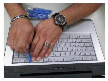
Locate plastic bezel above keyboard and use flat side of spudger to pry away from device.
