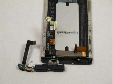
Pry back the speaker and microphone assembly from the bottom.
