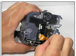
⚠ Before removing the LCD panel from the camcorder, disconnect the ribbon cables joining the LCD panel to the logic board.
