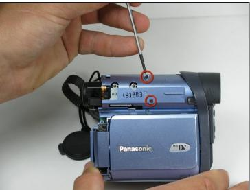
• Remove the indicated 4.5mm screws from the LCD side of the camera.
