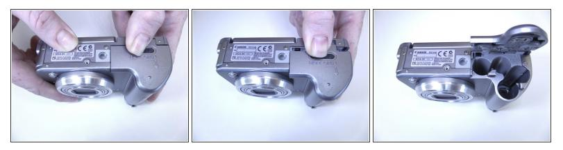
Slide the tab on the battery door while pushing the battery door away from you. The battery door should pop open.
