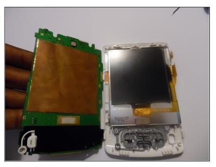
• Carefully remove the mother board by lifting up, exposing the keypad.
