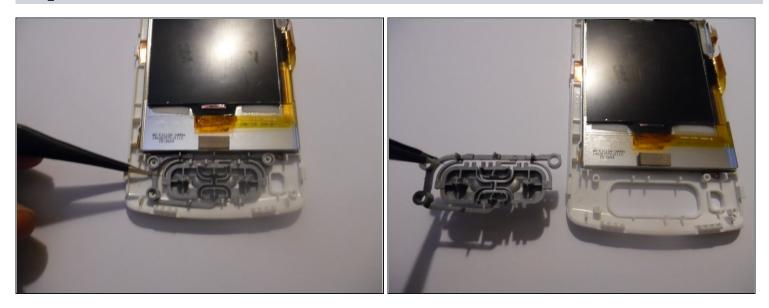
• Using tweezers, or something similar remove the keypad from the device and replace with a new one.
