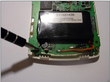
• Remove the two screws located at the bottom of the mothership, using a Philips head screwdriver.
