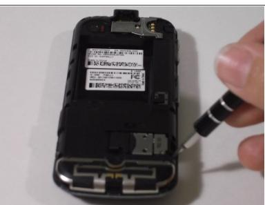
Remove eight black .4 centimeter screws on the top, bottom, and sides of the phone with a T5
