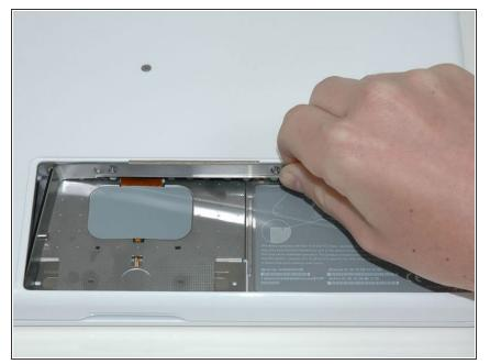
• Lift up on L-shaped memory cover, slide it to the right, and lift it out of the computer.
