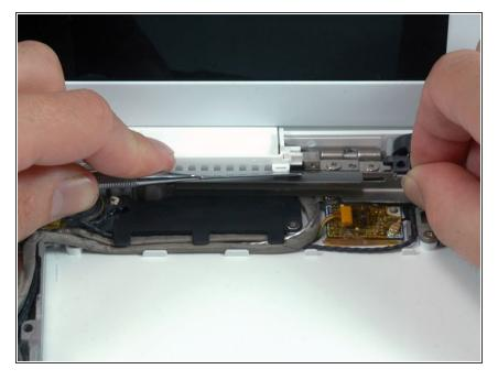
Using a spudger, gently pry up the white plastic slot and slide the metal c-channel to the right and away from the display.
