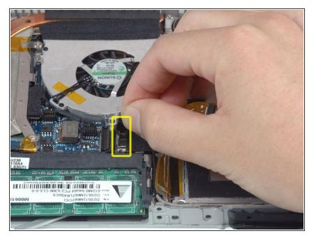
Disconnect the newly-revealed display data cable. If there is no pulltab on the top of the connector, it may be helpful to use a spudger to disconnect this connector.
