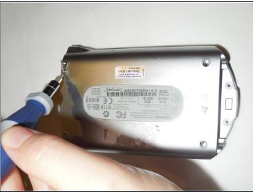
Remove the four 0.8mm Phillips # 00 screws from the back board using the screwdriver from your tool kit.
