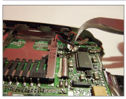
Detach the two pairs of wires, found on the top right of the motherboard, from their combs using the tweezers from the toolkit.
