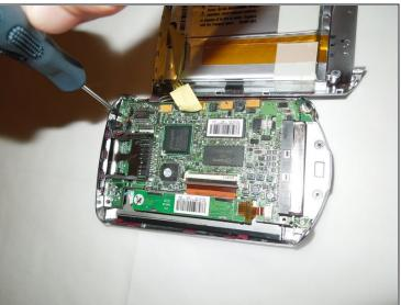
• Once the backboard is removed, remove the four screws on the motherboard. Two on top of the motherboard and two on the bottom of the motherboard using the Phillips screwdriver.
