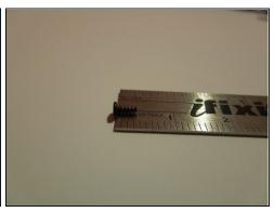
• Unscrew the two Phillips #00 screws to get the speaker loose using a Phillips screwdriver. The screws measure 0.3 mm in length.
