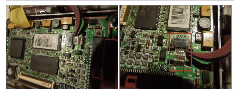
• In order to get to the speaker, try to free the motherboard by removing all the wires from their combs using the tweezers.
