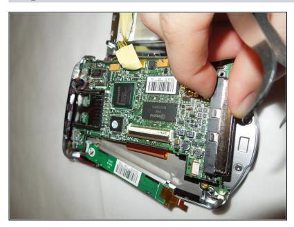
Once you have all the wires freed from the combs, you can detach the motherboard just by lifting it out of place.
