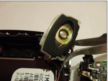
• Once the two screws that hold the speaker in place are removed, remove the speaker using tweezers.
